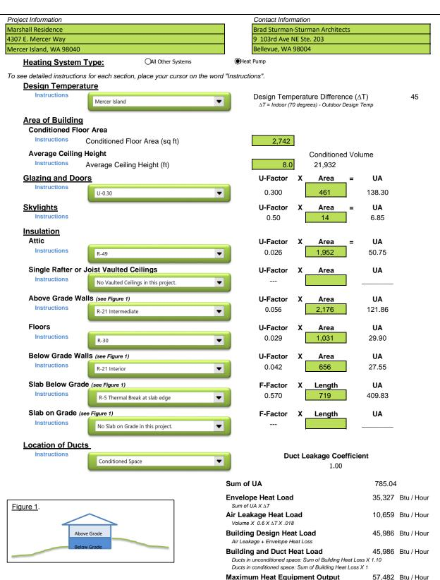
Building and Duct Heat Loss X 1.40 for Forced Air Furnace Building and Duct Heat Loss X 1.25 for Heat Pump
